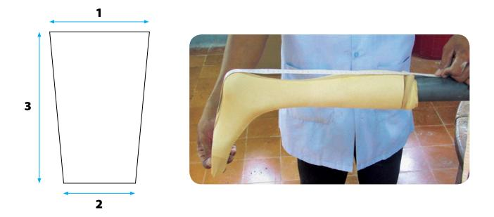
Heat the polypropylene at 180° for 20 to 25 minutes, depending on the thickness of the polypropylene and the efficiency of the oven.
