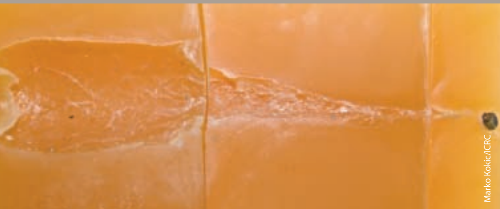
The track of a 7.62 mm semi-jacketed rifle bullet shot into a soap block.
