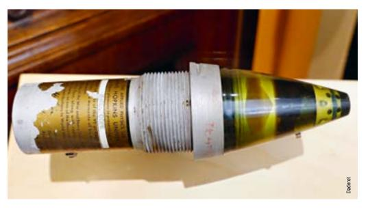
A proximity fuze is designed to detonate automatically at a specific distance from the target.
